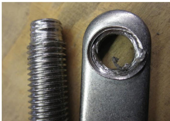
Galling is seizing or abrading of the threads, in which either the joint elements jam during the assembly or threads get damaged. It is also known as local cold welding (frictional bonding) of the thread flanks. It is generally formed when the thread flanks rub against each other for an extended period of time.
