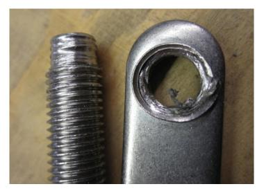
hen two fasteners are tightened together, surface pressure builds between the thread surfaces of the bolt and nut, and the protective oxide layer may break off. The high friction between the interfaces of
