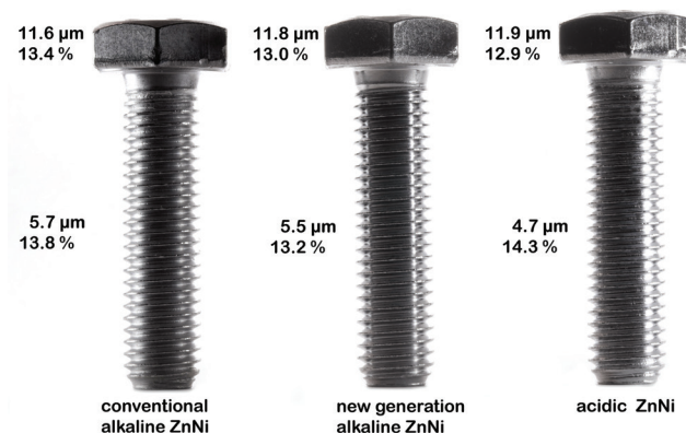
Figure 6: M8 x 40 bolt plated to the same thickness on the head (11.6μm – 11.9μm) in the three different zinc-nickel electrolytes: A conventional alkaline plating solution (left, ZINCROLYTE NCZ 315 Plus, 75 min plating time), newest development alkaline plating electrolyte ZINCROLYTE Sprint™ (middle, 50 min plating time) and the new generation acidic electrolyte ZINCROLYTE KCI-Ni IV (right, plating time 42 min). Minor differences in thickness distribution
